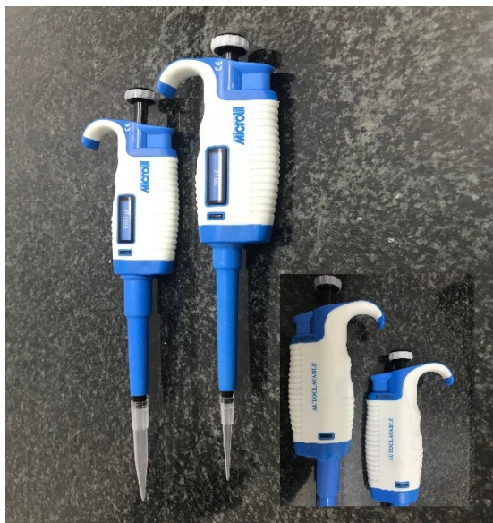
Single channel fixed micropipettes, nominal value: 20 µL and 1 000 µL
