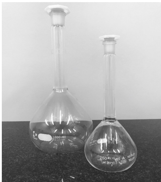
Single line glass flasks, nominal value 250 ml and 1000 ml
